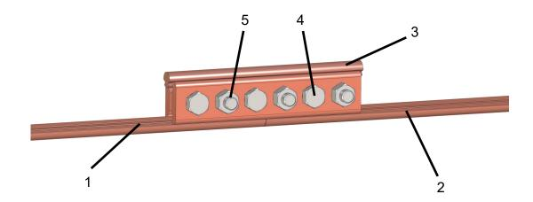
Splice fitting with piece of contact wire in the upper part.
