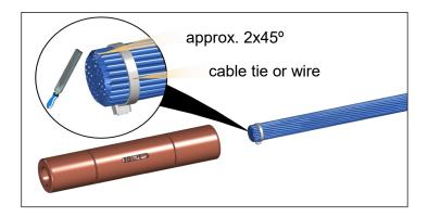
2. The cable should not be oxidized in the clamping part of the conical coupler. Oxidized cables should be cleaned with a wire brush.
