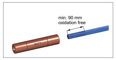
3. Insert the cable into the cone until it makes contact with the washer. The cable end must be visible through the window.
