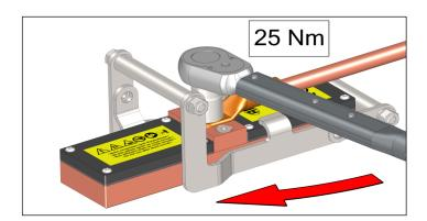
In order that the storage tube is always close to hand it is recommended that the earthing cable is passed through the tube before attachment to the magnetic earthing contact.
