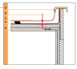
Wooden parapet with concealed drain.
