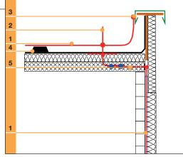
Wood balustrade with conductor cast in concrete.
