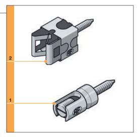
\*If the distance of 10 mm between the conductor and the flammable components of the building cannot be maintained, the minimal cross-section of this conductor must be 50 mm<sup>2</sup> on copper or 8 mm.
