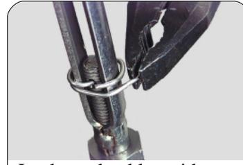
Lock turnbuckles with a locking wire.
