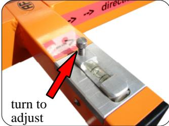
Place the JIG with red side to the installation direction. Adjust the spirit level for the red side.
