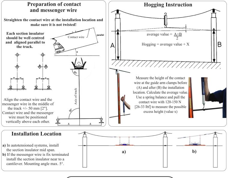
**! RISK OF DEATH !** Do not begin to work on the overhead line before you have ensured that it is switched off and correctly grounded!
