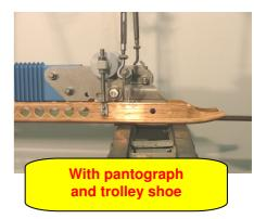
**24.** Readjust 3 droppers on either side to a straight downgrade line (if available)
