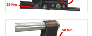
Perform an optical check if the entry splice is now level/parallel to the track. Use an adjustable spirit level or straight edge tool for the check.
