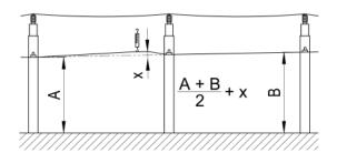
When replacing an existing section insulator measure the height of the contact wire at masts A and B. Calculate the average value. The hogging value should be minimum x = 70 mm.
