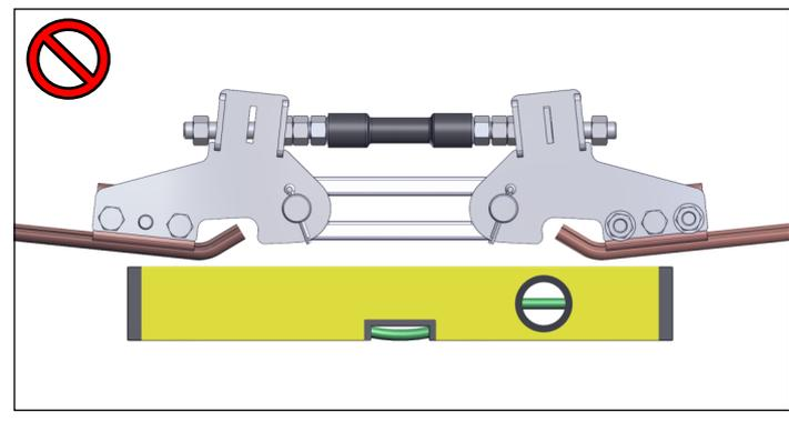
Counter the adjusting nuts with the counter nuts.
