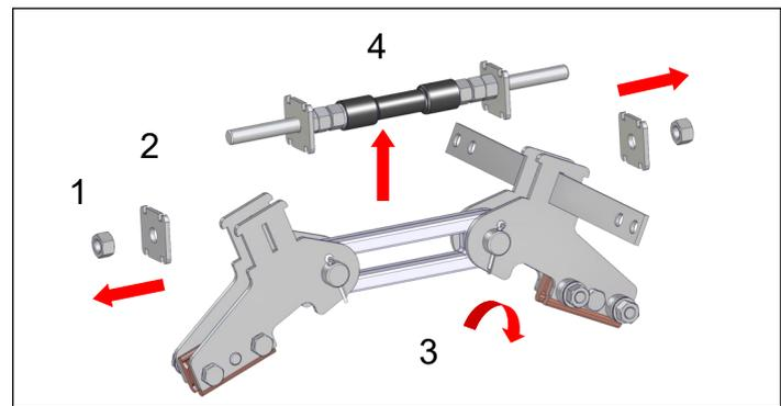
Remove the suspension plate.
