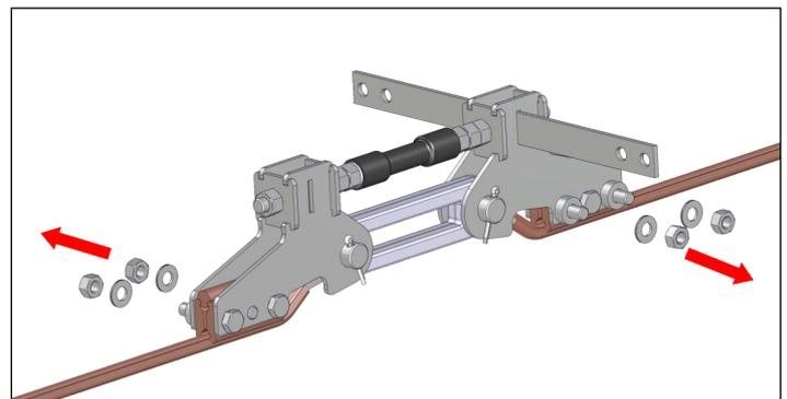
Install the runners to the insulator body using the locking washers and nuts.
