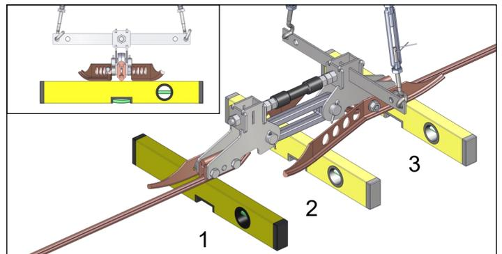
Tighten the nuts of the runners to **50 Nm** on both sides.
