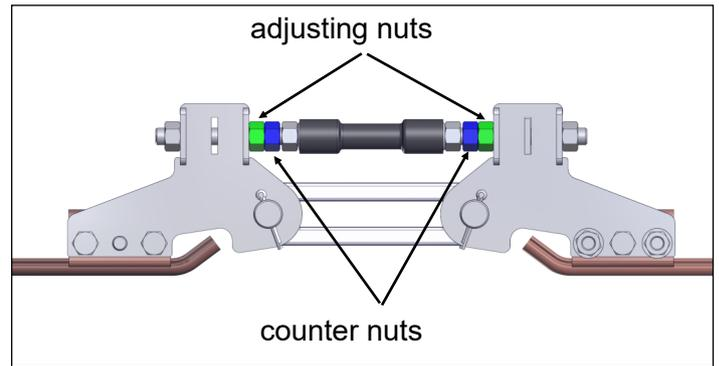
After aligning the isolator body, tighten the insulator nuts to **20 Nm**. Counter with the insulator hexagon nut.
