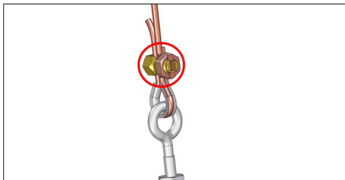
The tension in the two cable droppers must be the same.
