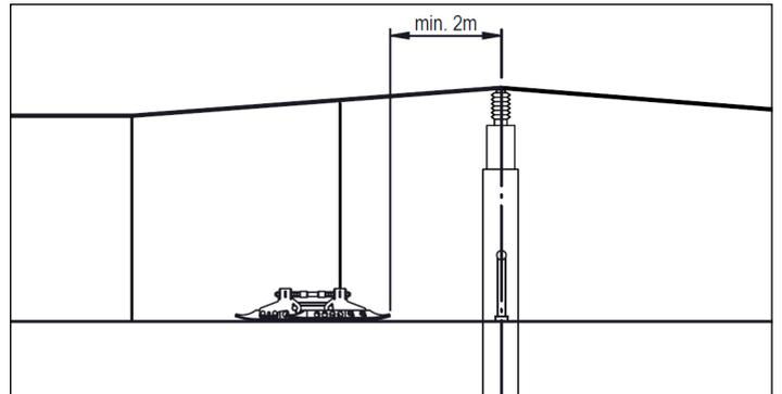
The sloping angle of the messenger wire should not exceed 5° if saddle clamps are able to glide.
