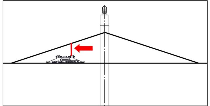
If the installation is done with messenger wire, the section insulator should be installed with a suspension and at least **2 m** away from the guide arm.
