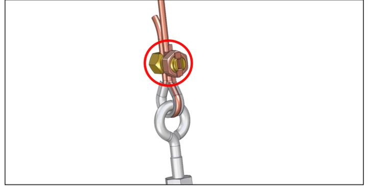
The tension in the two cable droppers must be the same.
