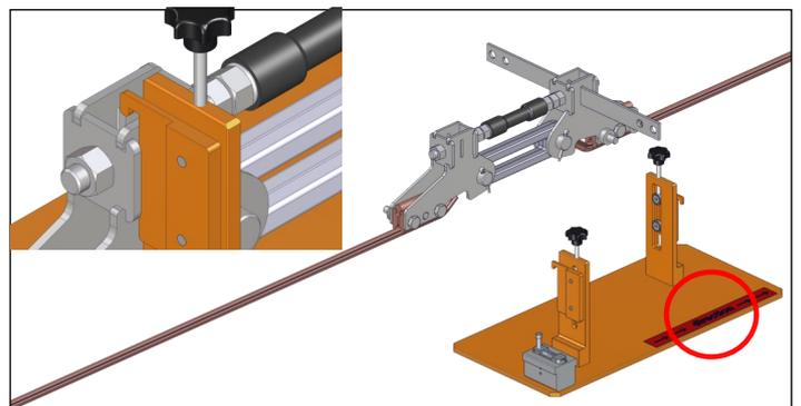
Tighten the grip screws of the installation JIG.
