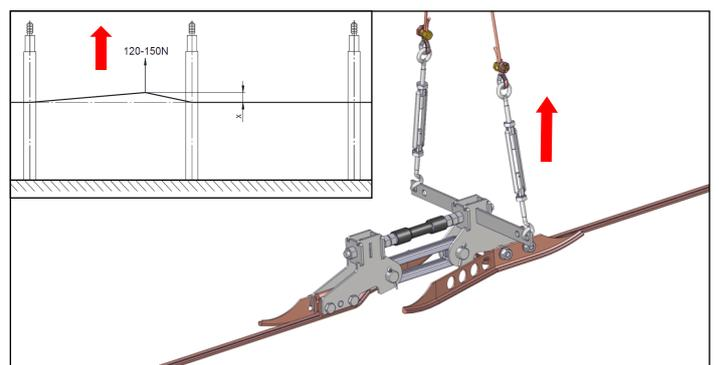
Tighten both cable dropper clamps to **25 Nm**.
