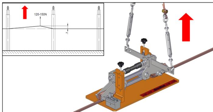
Tighten both cable dropper clamps to **25 Nm**.
