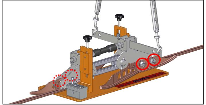
Remove the installation JIG by loosening the grip screws.
