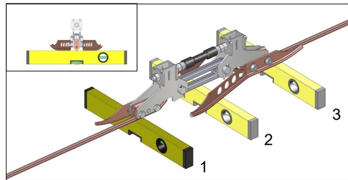
Tighten the nuts of the runners to **50 Nm** on both sides.
