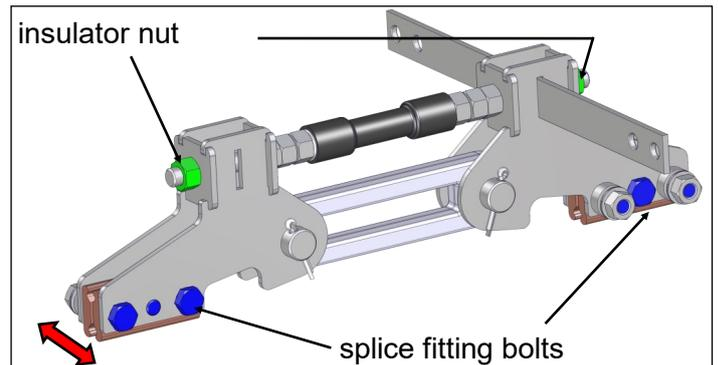
Insert a piece of contact wire in the upper part of each splice fitting.
